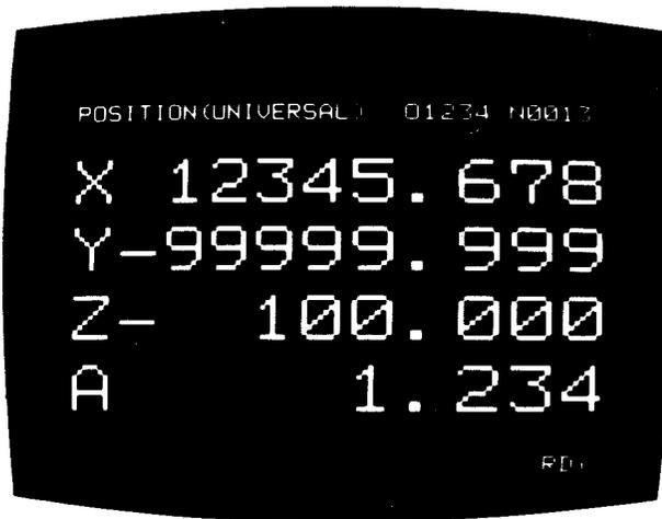
Fig. 4.20 Current Position Display ( External) -Example (with 4-axis control)
