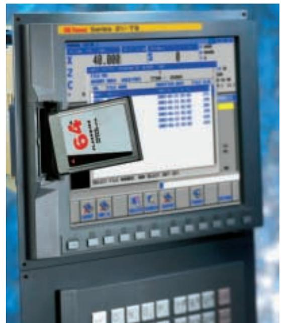
Workshop programming also has many friends, for which GE Fanuc offers special software. The highlight is the Manual Guide *i*. In version *i*, the developers have united the functionalities of the two predecessor versions, T (turning) and M (milling). With Manual Guide *i*, the user can now configure software for a turning, milling or compound machine.
